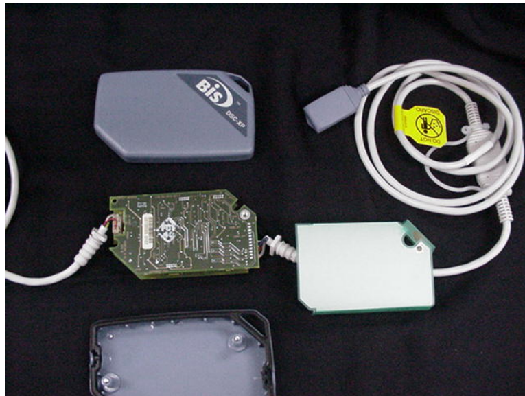
Figure 7-2 Remove the ground shield securing screw.
